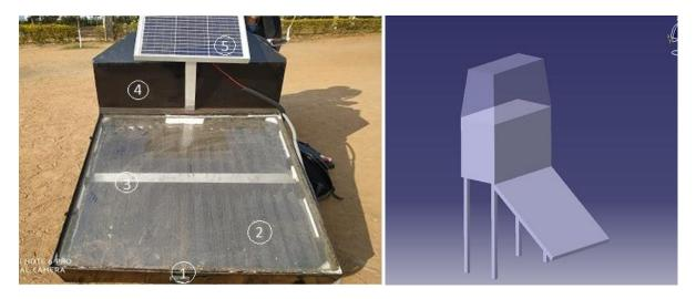
Figure 1. Experimental set up of front side of Hybrid type of Solar dryer.
