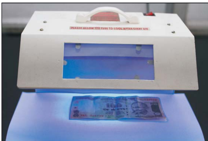
Figure 16.7: UV Lamp for Observing Fluorescence in Security Documents
