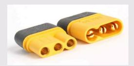
MR30 Connector : connector between DCU and atomizer
