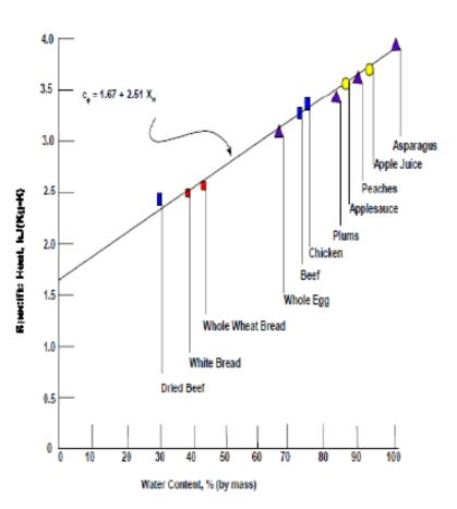
Figure 2.07. Specific heat of food products (at 0° to 20°C for meats, 4° to 32°C all others). Based upon ASHRAE data. (Courtesy of the American Society of Heating, Refrigeration and Air-Conditioning Engineers, 1989.)
