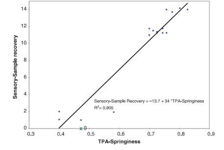
**Fig. 11.1** Linear regression and correlation between the sensory texture attribute sample recovery and the instrumental texture parameter springiness (TPA= texture profile analysis). Redrawn in a different orientation from Kim et al. (2009).
