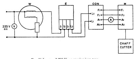
V = Voltmeter, 0.300 V, ac moving iron type E = Energymeter, 3 ampere, single phase, 1 600 rev/kWh W = Wattmeter, 0.230 V, single phase, dynamometer type CON = 1.5 kW speed controller M = dc motor shunt wound, 1.5 kW, 220 V A = Ammeter, 0.10 AFIG. 1 CIRCUIT DIAGRAM
