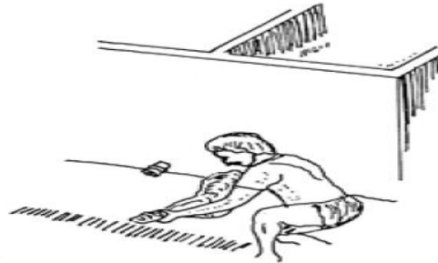
b. install bag net outside drain pipe; open drainage
