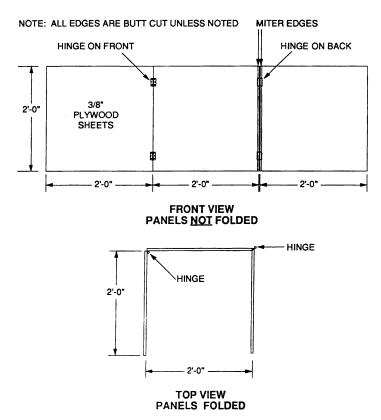
**Fig. 3.1** Construction information for portable sensory booths.
