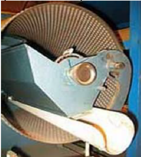
Working principle of the indented cylinder separator
