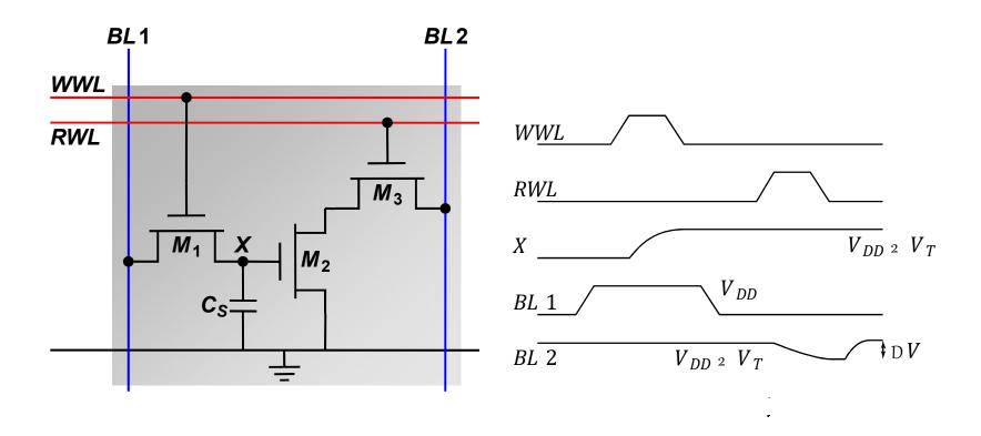
No constraints on device ratios Reads are non-destructive Value stored at node X when writing a "1" =  $V_{WWL}$ - $V_{Tn}$
