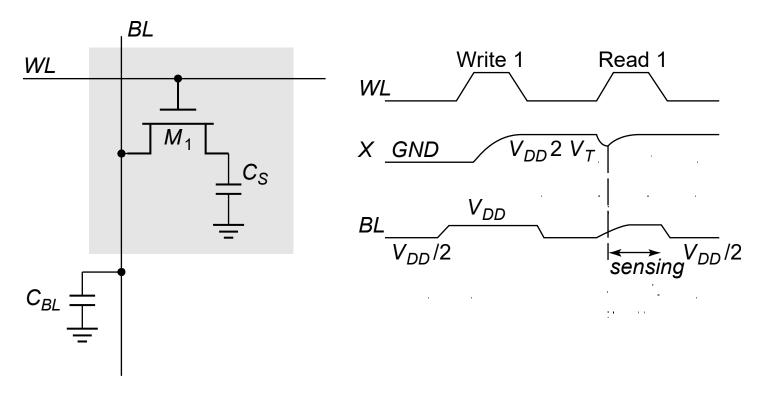
Write: C<sub>S</sub> is charged or discharged by asserting WL and BL.
