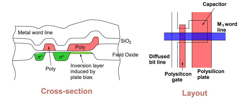
Uses Polysilicon-Diffusion Capacitance
