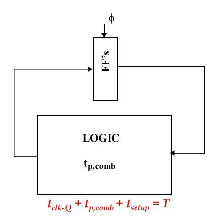
Also:  $t_{cdreg} + t_{cdlogic} > t_{hold}$  $t_{cd}$ : contamination delay = minimum delay
