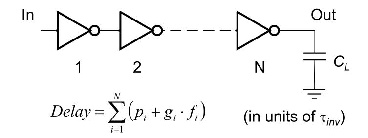
For given *N*:  $C_{i+1}/C_i = C_i/C_{i-1}$ To find *N*:  $C_{i+1}/C_i \sim 4$ How to generalize this to any logic path?
