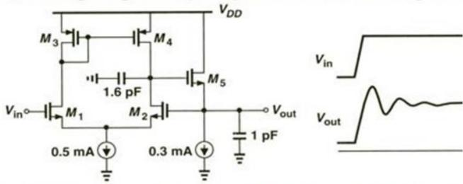
The large-signal step response of feedback amplifiers is n slewing but also because of the nonlinear behavior result excursions in the bias voltages and currents of the a excursions in fact cause the note and zero frequencies to p
