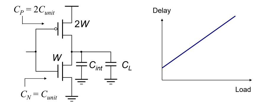
Delay =  $kR_W(C_{int} + C_L) = kR_WC_{int} + kR_WC_L = kR_WC_{int}(1 + C_L/C_{int})$ = Delay (Internal) + Delay (Load)
