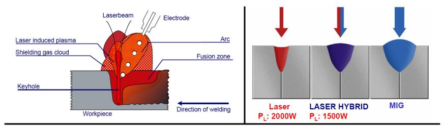
ARC Low-cost energy source Gap bridgeability Microstructure can be influenced
