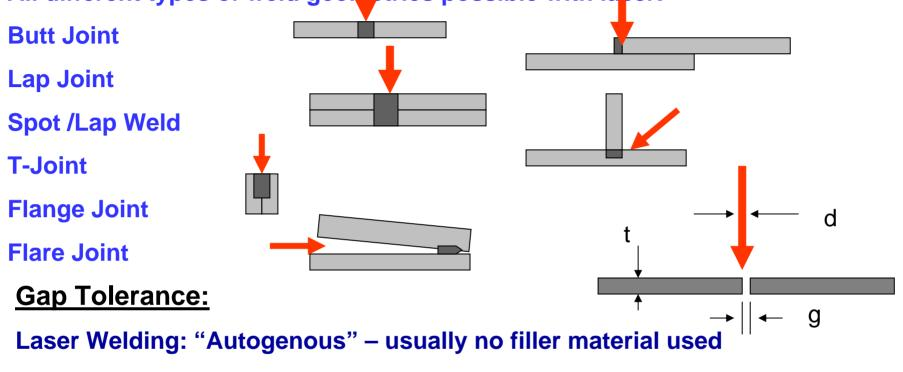
Gap between two parts: Less than half of the laser beam diameter for efficient laser power coupling, g < 0.5d
