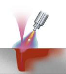
LASER High penetration High welding speed Low heat input High tensile strength
