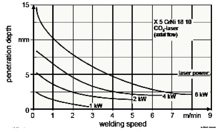
1 kW of laser power per mm thickness is needed to weld at 1 m/min.
