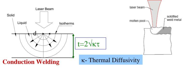
τ- Laser Interaction Time = Laser pulse duration = Laser dwell time = Beam diameter d/Welding speed v
