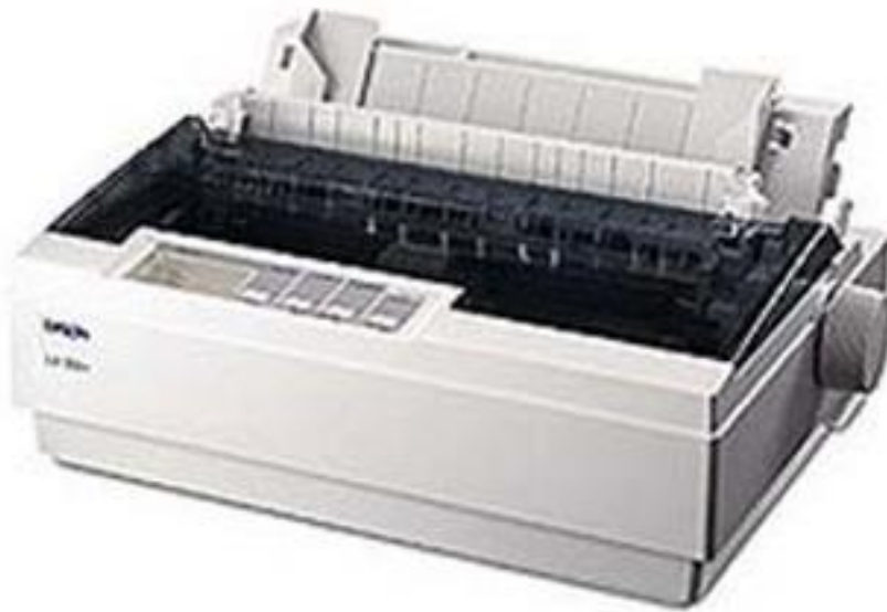
Fig. 15-3 This Printer is used for alarms for a process. Each alarm was recorded at the time of occurrence and printed as a single line of data to be analyzed by a process engineer or controls engineer.
