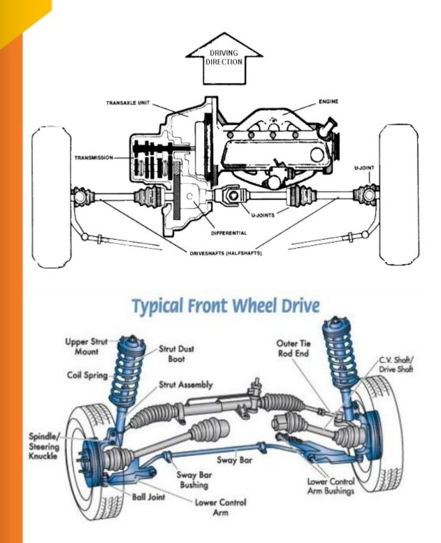
During acceleration of the vehicle or during braking, the torque reaction causes the engine to rotate about the crankshaft. Hence engine mountings are suitably located and secured to resist this movement. The thrust and braking torques are borne by the suspension members especially the tie bar joining the track control arm to the body.
