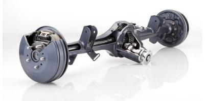
b) Split or Salisbury Type Axle: This type of axle is more rigid than a banjo type and is often employed to support a hypoid gear. The final drive assembly is installed in a rigid malleable cast iron carrier or housing, into which the axle tubes are pressed and welded. For extra rigidity reinforcing ribs extend from the pinion nose to the main carrier casing. A domed plate is fitted at the rear of the casing to provide access to the final drive gear.
