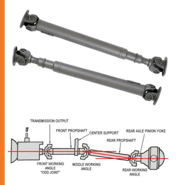
This shaft must be strong to resist the twisting action of the driving torque and it should be resilient to absorb the torsional shocks. It must resist the natural tendency to sag under its own weight because vibration occurs when the centre of gravity does not coincide with the axis of the shaft.
