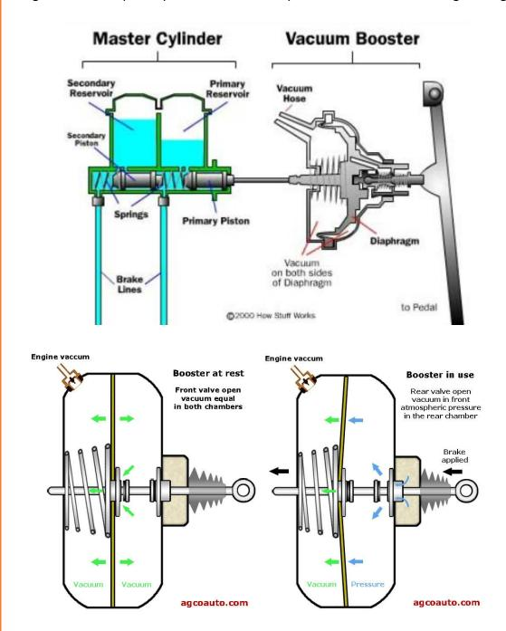
Schematic layout of a vacuum brake booster is shown above.
