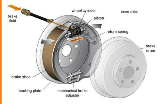
A **drum brake** is a brake that uses friction caused by a set of shoes or pads that press outward against a rotating cylinder-shaped part called a brake drum. The shoes are stationary while the brake drum carries the wheels and rotates along with the wheel hub (front and rear).
