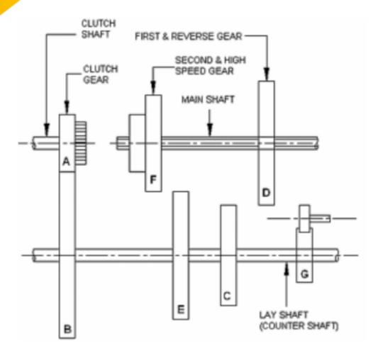
Shafts – Sliding mesh gearbox consists of 3 nos. of shafts which are: -
