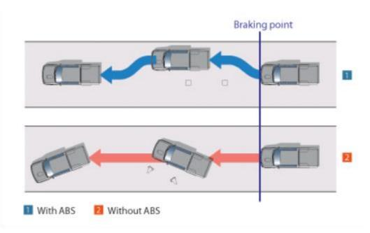
It is difficult to assess the required brake pedal force to be applied for an emergency stop in the shortest possible distance. This is because it is practically impossible to consider several varying factors such as: -
