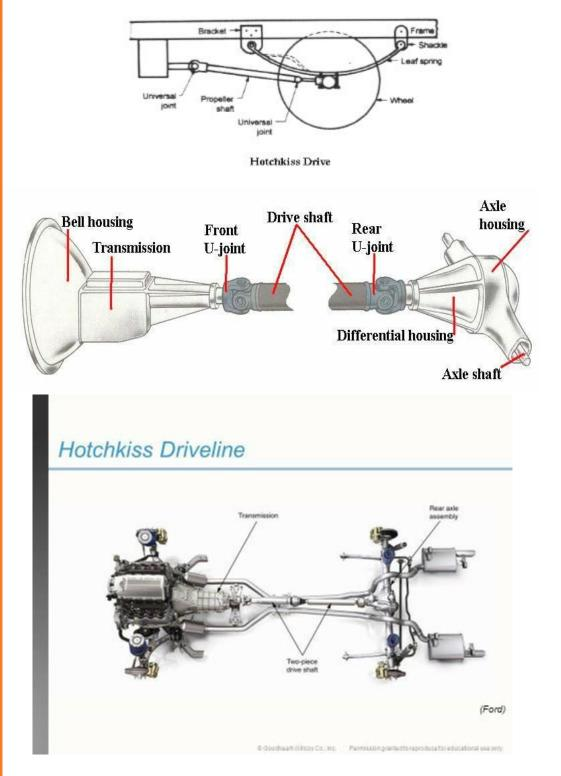
The arrangement uses two rear leaf springs, which are longitudinally mounted and are connected to the chassis frame by a "fixed" pivot at the front and swinging shackles at the rear. A universal joint is mounted at each end of the exposed or "Open type Propeller shaft" with provision for accommodating change in shaft length due to the deflection of the springs through a slip joint.
