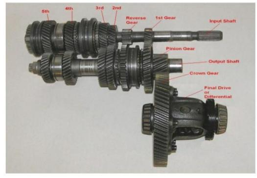
The power flow through the transmission section of the transaxle is the same as through a conventional transmission.
