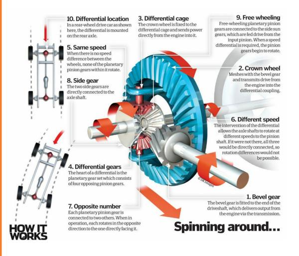
During movement of the vehicle on straight, level road and with both tires having equal traction (traction means adhesive or pulling friction of a tire on the road), there is no differential action. In this case, the crown wheel, differential case and cover, differential pinion gears and the differential sun gears all turn as one unit. The differential pinion gears do not rotate about their axis on the spider but rather turn both the sun gears and axle shafts at the same speed.
