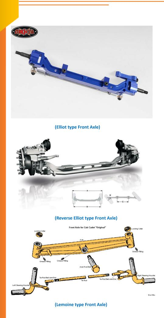
In a "Dead Front Axle", the front wheel hubs are supported on bearings at the end of the stub axles. During movement of the vehicle, the front wheel hubs freely rotate on these bearings. The stub axle is attached to the steering linkages vide which they can be turned left or right as per requirement.
