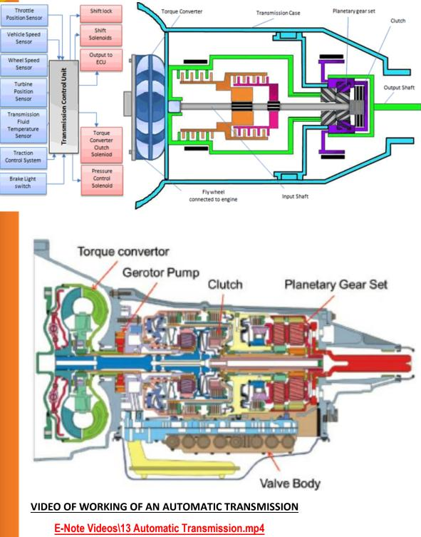
Schematic layout of an automatic transmission is shown below: -
