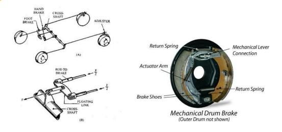
The layout of a simple mechanical brake system is illustrated in **Fig. A** above. Four adjustable rods or cables connect the brake shoe operating levers to a transversely mounted cross-shaft. The footbrake and handbrake controls are connected to the cross-shaft using links with elongated holes that allow independent operation of each control.
