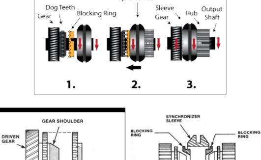
Gear shoulder and blocker ring mating surfaces.
