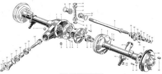
Fig. J.1. REAR AXLE-COMPONENTS.
