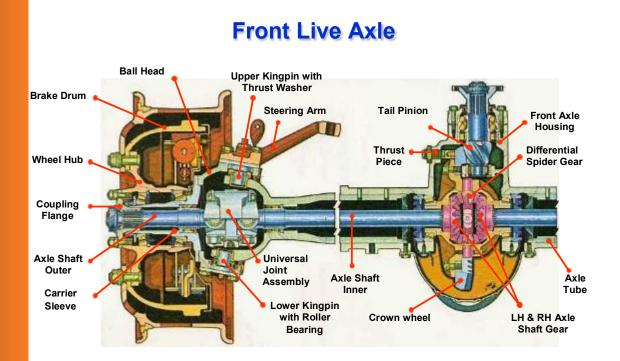
The front axles are generally dead axles, which does not transmit power. The front wheel hubs rotate on antifriction bearings of tapered-roller type on the stub axles. To permit the wheels to be turned by the steering gear, the steering spindle and steering knuckle assemblies are hinged on the end of the stub axles. The pin that forms the pivot of this hinge is known as king pin or steering knuckle pin.
