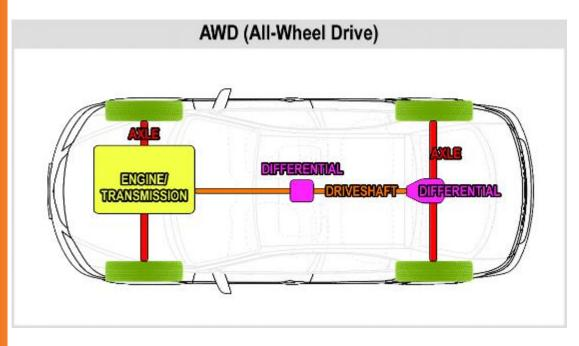
Other AWD vehicles have front-wheel drive with auxiliary rear-wheel drive, or rear-wheel drive with front wheel drive. Some AWD vehicle have a single speed transfer case. Others have the gearing to drive the auxiliary axle built into the transmission or transaxle.
