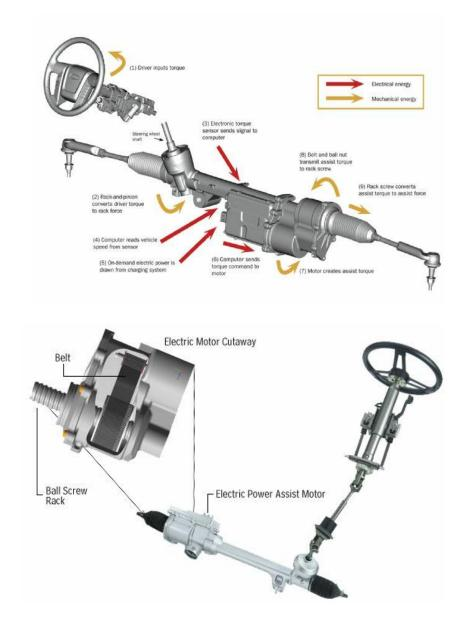
Pictures above shows the construction and operation of an electric power assisted steering mechanism.
