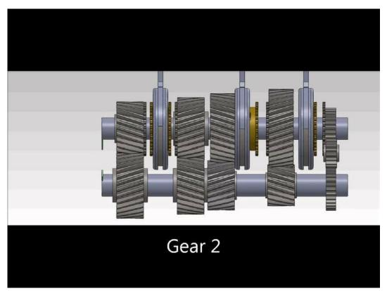
• Power Flow Diagram in a 5-Speed Synchromesh Gear Box
