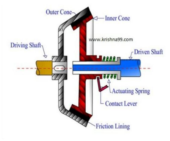
Principle of Operation of Cone Clutch:
