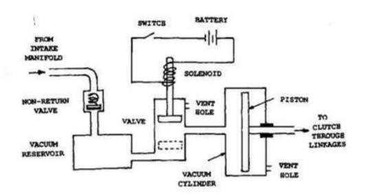
In the normal position,3 the switch in the gear lever remain open and the solenoid operated valve remains open (shown by the dotted position). At this stage, the pressure on both sides of the piston in the vacuum cylinder is atmospheric since the vacuum cylinder is open to the atmosphere through a vent. When the switch is closed due to the operation of gear change
