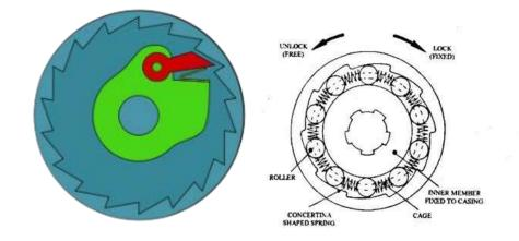
A more sophisticated and rugged design has spring-loaded steel rollers inside a driven cylinder. Rotating in one direction, the rollers lock with the cylinder making it rotate in unison. Rotating slower, or in the other direction, the steel rollers just slip inside the cylinder.
