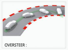
Rear tires lose grip and causing the rear end of the vehicle slides out. Oversteer can be corrected by stiffening the vehicle's front chassis.
