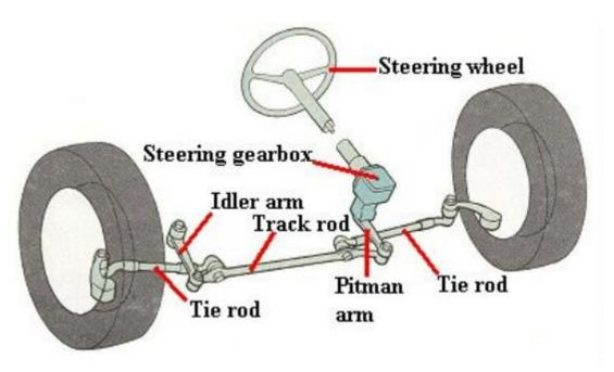
The steering system allows the driver to control the direction of vehicle travel. This is made possible by linkages that connects the *steering wheel* to the steerable wheels and tires. To increase the mechanical advantage of the rotary motion of the steering wheel to liner motion, a *steering gear box* is provided between the steering wheel and the linkages as shown above.
