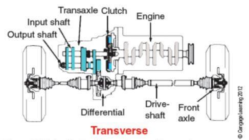
Figure 77.4 A side-to-side engine and transaxle.
