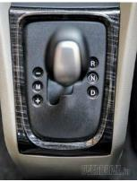
R: Reverse, N:Neutral, D: Drive, M: Manual, +/- : Gear shift in Manual mode
