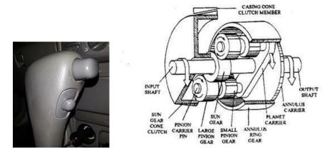
To transmit power in overdrive gear train, the sun gear is held stationary, and the input shaft and planet carrier are rotated. This forces the large planet gear
