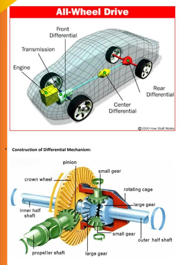
The differential mechanism consists of following components: -
