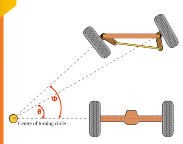
In order to avoid tire slippage when a vehicle takes a turn, it is necessary that each wheel must roll on an arc which has a common center with arcs of other wheels of the vehicle as shown above. This condition is called as "Pure rolling". To satisfy the situation of pure rolling, following conditions must be satisfied: -
