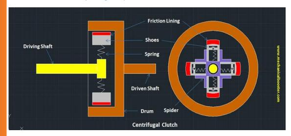
Main parts of a Centrifugal clutch are: -
