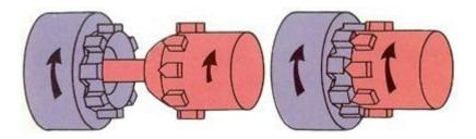
The outer surfaces of the shafts are splined, one side carrying an internally splined collar; when the speeds have been synchronised by the cones, the splines may still not be aligned, so those on the collarless side are pointed to facilitate engagement.
