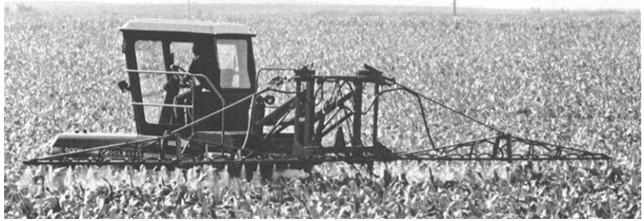
Figure 10.20 – A boom-type field sprayer (reproduced by permission of Deere and Co., © 1991. All rights reserved).
