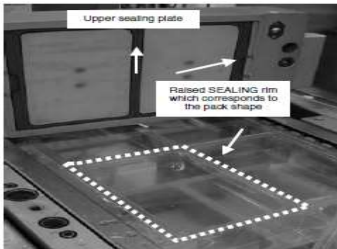
Figure 10.10 Top web heat sealing on the Multivac R230.
