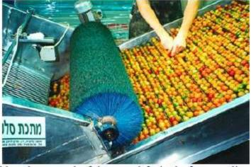
Fig.4: Brushing and hand removal of damaged fruits before grading
