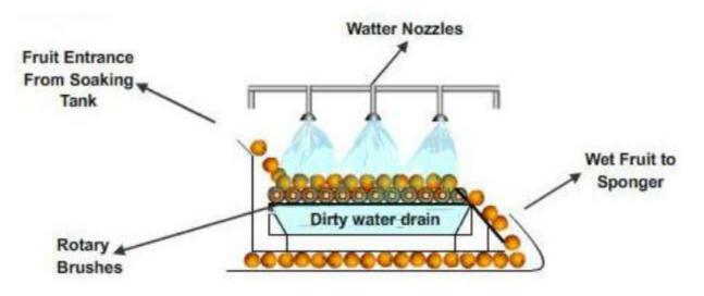
Fig.: A typical fresh produce washing machine
