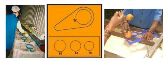
Fig.:11 Sizing with rings of known diameters
